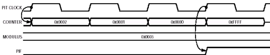
Figure 16-6: Counter in Free-Running Mode
